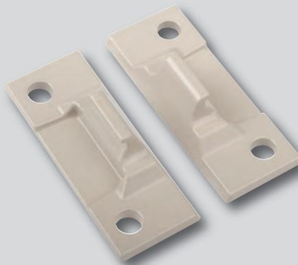
*High Performance Snubber* - Concealed within the hinge cavity, Truth's new High Performance Snubbers help create a better seal and increases negative air pressure performance (achieving a minimum of 350 lbs of negative air pressure) when a pair of snubbers are used.
