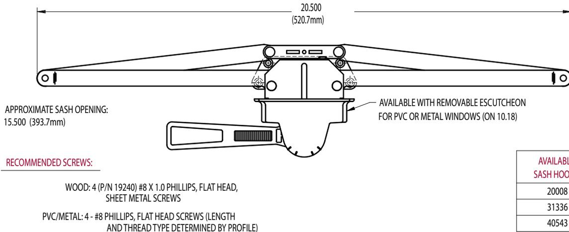
**FIG. 3 DUAL PULL LEVER OPERATOR 10.11 (removable escutcheon 10.19)**
