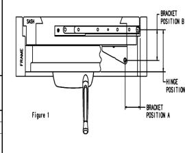
The maximum window size, ease of operation, and service life are strongly influenced by hardware mounting positions (see Fig. 1 below).
